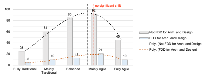
Fig. 3. Integrated histogram for the project discipline Architecture and Design (n=536) and for the method Feature-Driven Development (n=59) within the Architecture and Design discipline (note that, even though we illustrate this as a curve, the applied test works on categorical data)
